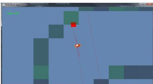
Figure 5: AI raycasting from the centre of the car
