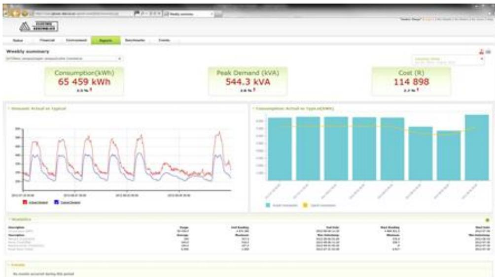
**Fig. 1.** A screen grab of the dashboard showing energy data for eight days
