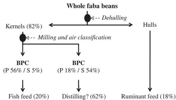
**Figure 2.** A schematic diagram of the possible fates of fractioned whole faba bean components following air classification. The percentages denote proportions of the faba bean starting weight. P and S denote protein and starch content (%), respectively. [BSC = bean starch concentrate; MBG = malted barley grist]
