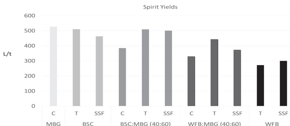
**Figure 3.** Potential spirit yields from faba wort fermentations calculated on basis of starch content
