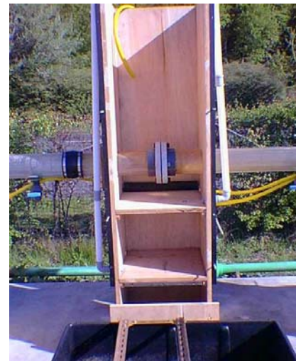
Figure 2. View of interior of test box before addition of gravel showing pipe joining structure
