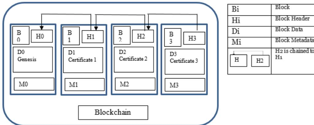
Figure 7. The blockchain components of the proposed system
