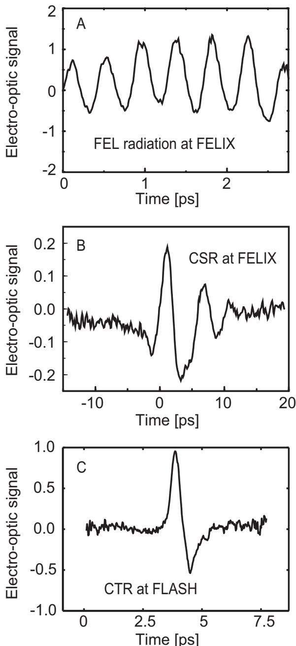
Figure 3: Single-shot electro-optic measurements of (A) FEL radiation, (B) CSR radiation and (C) CTR radiation. The leading edges of the pulses are on the left. Note the different time scales. See text for details.
