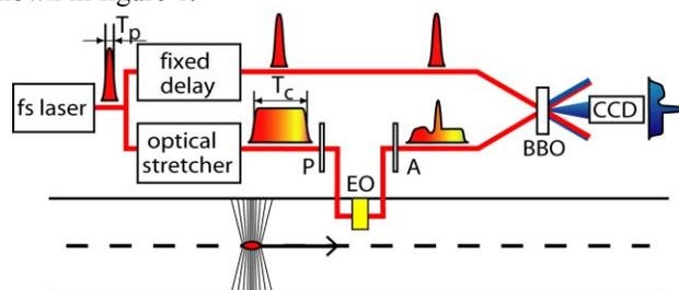
Figure 1: The single-shot technique for measuring the longitudinal electric field profile of electron bunches using electro-optic encoding and temporal decoding. P and A are polarizers, BBO is the second-harmonic crystal of the cross-correlator and the signal is recorded by the CCD.
