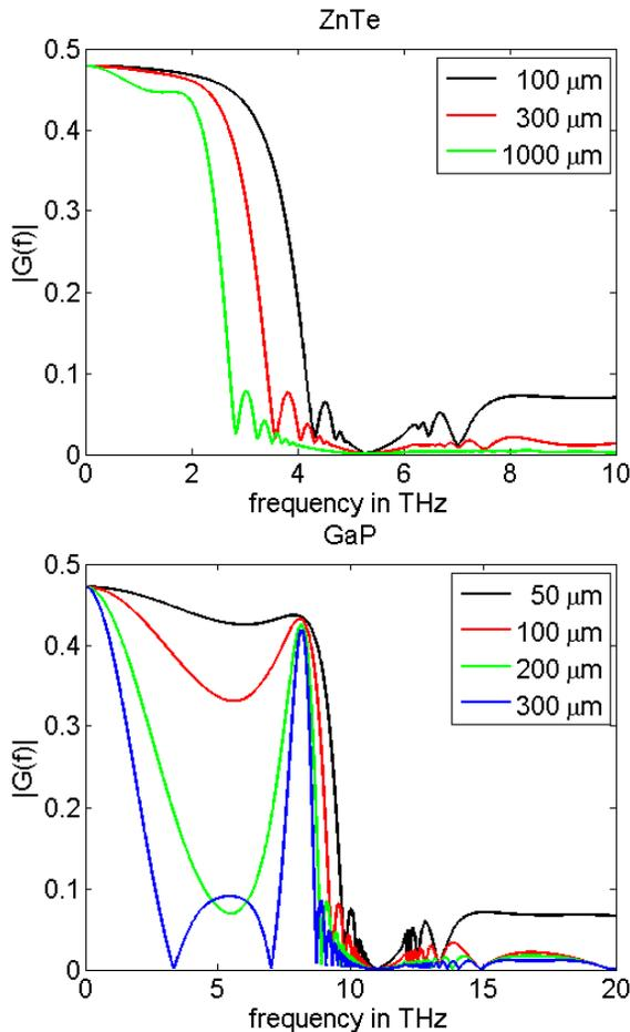
Figure 2: Electro-Optic response function for ZnTe (upper) and for GaP (lower) for different thickness of crystal.
