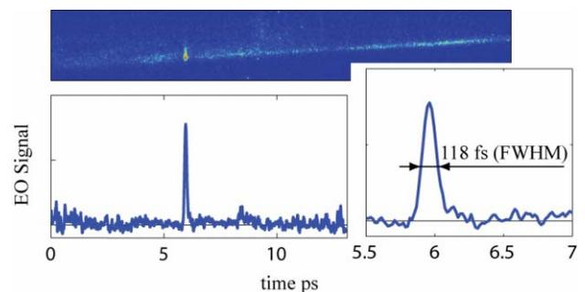
Figure 3: A typical measurement from temporal decoding showing the camera image and a binned image. The insert displays an exploded view of the peak.
