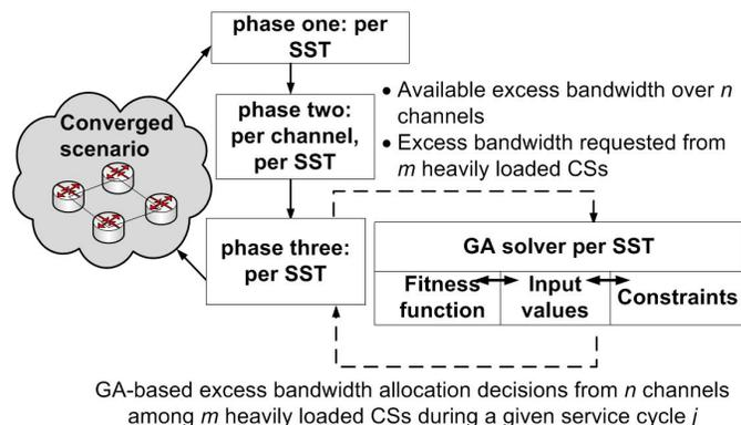
Figure. 1 The GA-based framework for dynamic excess bandwidth allocation algorithm
