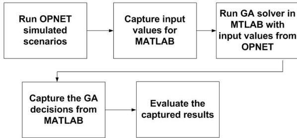
Figure. 2 Employing the GA solver for the input values from the OPNET converged scenarios
