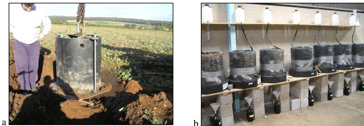
Figure 4. Soil core collection (a) and leaching study (b)
